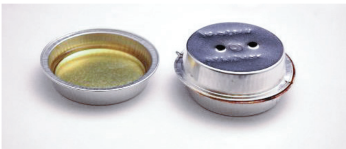
Test is performed using a capped dish simulating the chain's working conditions
